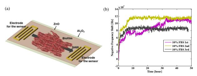
Fig. 3: (a) A schematic of the SAW sensor, (b) Resonant frequency shift results in three consecutive *E. coli* biofilm growth experiments in an animal serum (10% Fetal Bovine Serum) [4].
