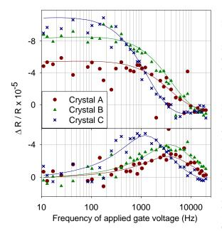
**Figure 2** The infrared response measured as a function of the frequency of the gate voltage. The y-axis shows the change in reflectance of the transistor,  $\Delta R = R_{on} - R_{off}$ , normalized to the total reflectance both in-phase (top-panel) and in quadrature (bottom panel) with the applied voltage. Measured mobilities are 0.13, 0.12 and 0.07 for crystals A, B, and C, respectively.
