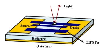
**Figure 1** Cartoon of a TFT with TIPS Pn as the active material. Also shown is the approximate size of the infrared light measurement area.
