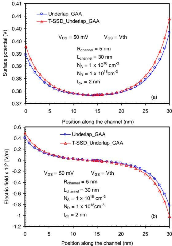
Figure.2 (a) Variation of surface potential as a function of position along the channel of T-SSDE Gate Underlap GAA MOSFET. Fig. (b) Variation of electric field as a function of position along the channel of T-SSDE Gate Underlap GAA MOSFET, Channel length  $L = 30$  nm, Diameter of Si pillar  $t_{si} = 10$  nm, work-function of the metal gate electrode  $\Phi_m = 4.8$  eV (optimized), dielectric permittivity of  $\text{SiO}_2$  is  $\epsilon_{ox} = 3.9$ .
