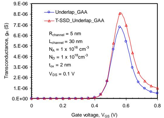
Figure. 5 Variation of transconductance ( $g_m$ ) as a function of applied gate bias ( $V_{GS}$ ) at applied drain voltage ( $V_{DS} = 0.1$  V) of T-SSDE Gate Underlap GAA MOSFET,  $N_A = 1 \times 10^{16} \text{ cm}^{-3}$ ,  $N_D = 1 \times 10^{18} \text{ cm}^{-3}$ ,  $\text{SiO}_2$  thickness  $t_{ox}$ , work-function of the metal gate electrode  $\Phi_m = 4.8$  eV, dielectric permittivity of  $\text{SiO}_2$  is  $\epsilon_{ox} = 3.9$ .
