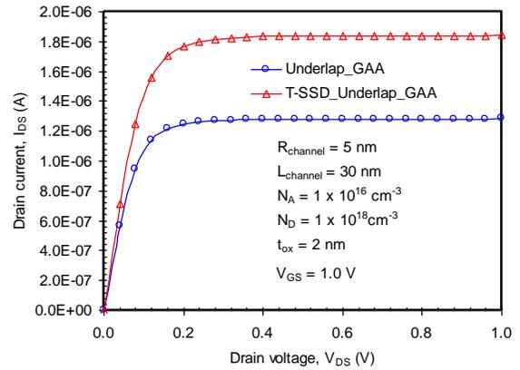
Figure. 4 Variation of drain current ( $I_{DS}$ ) as a function of applied drain bias ( $V_{DS}$ ) at applied gate voltage ( $V_{GS} = 1.0$  V) of T-SSDE Gate Underlap GAA MOSFET.
