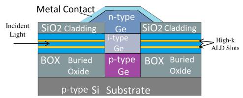
Fig.1. Schematics of the waveguide-detector junction. The detector mesa is grown after fabrication of the waveguides. A PIN diode is formed using epitaxy. The incident light will face the intrinsic germanium to maximize the quantum efficiency.
