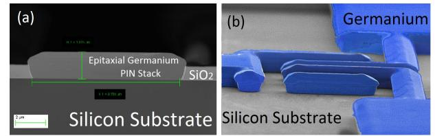
Fig.3. (a) Cross section SEM micrograph of the selectively grown PIN junction. (b) SEM image of grown germanium extruded features using selective epitaxy.
