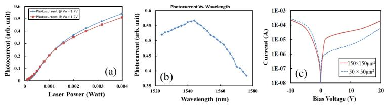
Fig.4. Shows the photocurrent measurements versus (a) laser power at 1.2V and 1.7V bias, and (b) laser wavelength at 1.2V bias. (c) Shows the current measurements in darkness.
