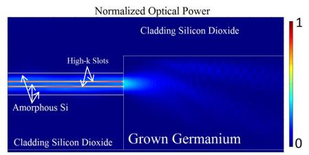
Fig.2. Simulated wave propagation profile representing the normalized optical power. Coupling of the guided mode into the germanium active region is demonstrated. High optical mode confinement can also be observed in the slot regions. The circuit is designed for the TM mode.
