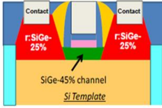
Fig. 1. Schematic diagram of the SiGe channel MOSFET with raised SiGe source/drain region in this work. The material for the channel is \text{SiGe}_{0.45} , with \text{SiGe}_{0.25} for the source/drain. After [3].
