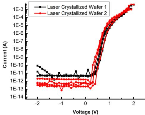
Figure 3: IV characteristics of laser crystallized diodes. Squares and circles show multiple devices on two wafers.
