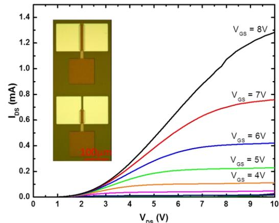
Figure 1: SLS transistors with grain boundaries parallel to current conduction. W/L=100/20,  $\mu$ ~450 cm<sup>2</sup>/Vs, V<sub>T</sub>~1.7 V. Inset shows micrograph of completed laser crystallized transistors.
