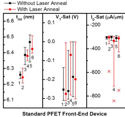
Figure 4: Front-end transistor parameters ( $t_{ox}$ ,  $V_{T-Sat}$ ,  $I_D-Sat$ ) for NFET and PFET devices. Each line plots the maximum, minimum, and median of twenty measurements. Overall, except for possible processing issues in p-channel wafer 4, the laser crystallization process does not have any measurable effect on front-end characteristics.
