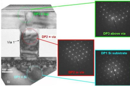
Figure 2: Bright field TEM image and electron diffraction images showing each region with high degree of crystallinity and having the same crystal orientation as the silicon wafer.
