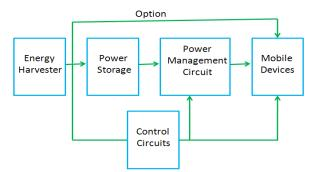
Figure 2 Scheme for power solutions suitable for nodes of WSNs.
