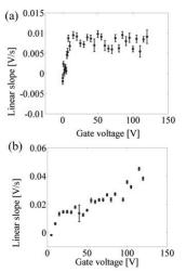
Figure 2: Trap formation rate versus gate voltage for (a) dEO PDI on bare  $SiO_2$  transistor channel and (b) dEO PDI on HMDS-treated  $SiO_2$  transistor channel.
