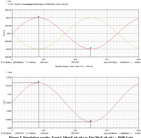
Figure 3. Simulation results: Vout(1.156mV pk-pk) vs Vin(20µV pk-pk) = 35dB Gain
