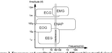
Figure 2. Frequency and amplitude ranges of different biopotential signals [2]
