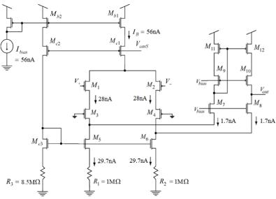
Figure 1. Low Power (107nW) Neural Amplifier [1]
