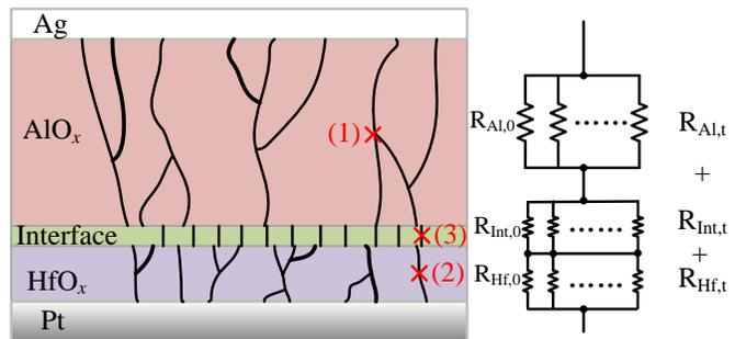
Fig. 6 Schematic of proposed switching model for stack layers in 4# RRAM devices.
