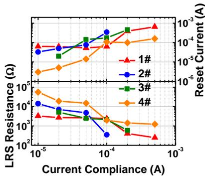
Fig.3 Maximum reset current and LRS resistance as a function of the current compliance.
