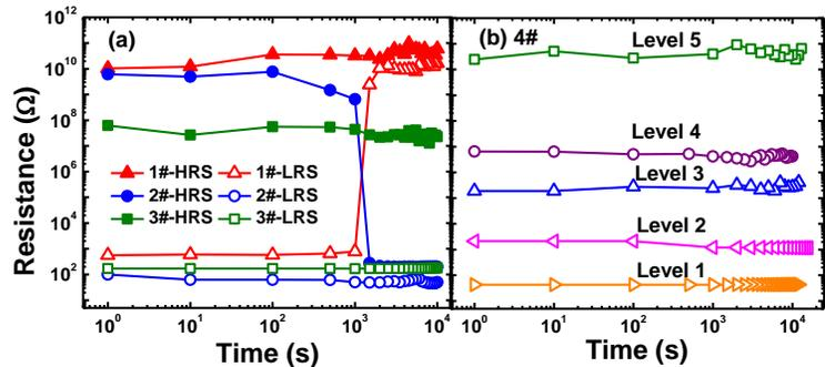
Fig. 5 (a) Retention performance of 1-3# RRAM devices and (b) Multi-level retention performance of 4# RRAM devices.
