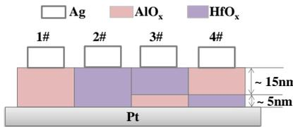
Fig.1 Schematic structure of 1-4# RRAM devices.
