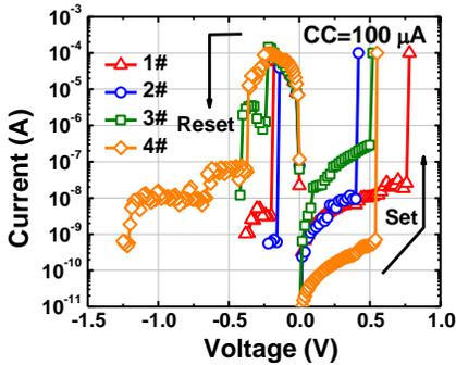
Fig.2 Typical current versus voltage (I-V) curves of 1-4# RRAM devices.
