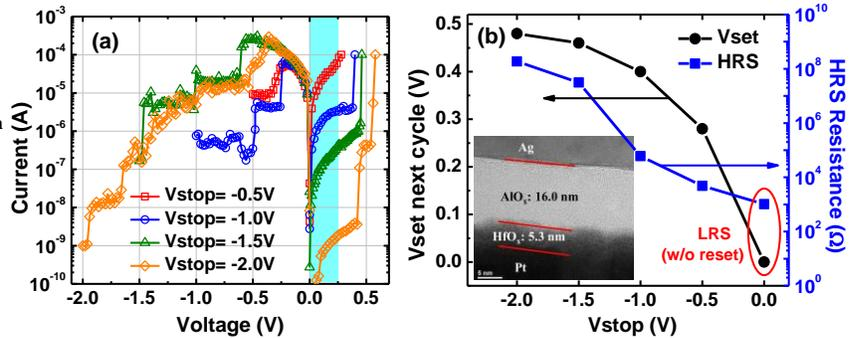
Fig.4 (a) Multi-level storage realization controlled by reset voltage in 4# devices. (b) HRS resistance and set voltage in next DC cycle as a function of reset voltage. The inset is HRTEM image of 4# stacked layers.
