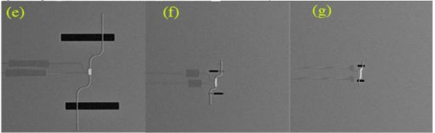
(e), (f) and (g) are images of 300 GHz, 1 THz, and 3 THz devices, respectively. A thin layer of Bi is deposited to act as an radiation absorber.
