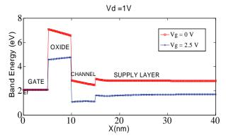
Figure 6: Band diagram along the depth of the device at its medium
