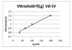
Figure 4: Change in threshold voltage  $V_T$  as Lg increases.
