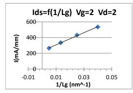
Figure 5: Variation of the current -standardized at Vd=Vg=2V-as the gate length Lg decreases.
