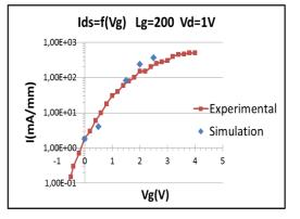
Figure 2: Variation of current with gate voltage Vg (solid line) contrasted to experimental values.
