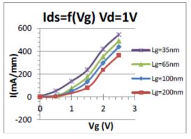
Figure 3: The variation of the current Ids as a function of Vg for different gate lengths.
